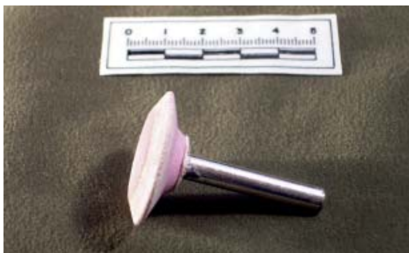
Fig. 14 A modern abrasive tool used to make the slit cavity in soft stones.
